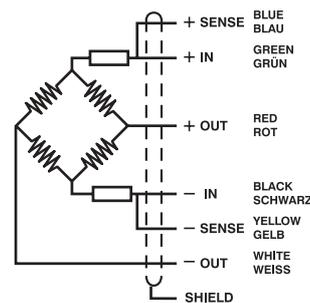
«SENSES»: 2 additional wires to maintain a constant voltage supply at the load cell when used with proper instrumentation. Use specially when long wires and wide temperature range.
