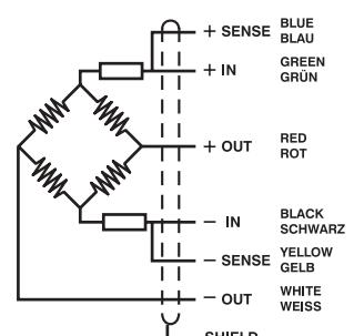
«SENSES»: 2 additional wires to maintain a constant voltage supply at the load cell when used with proper instrumentation. Use specially when long wires and wide temperature range.
